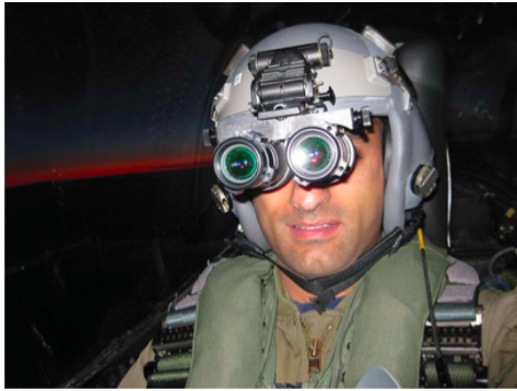
FIGURE 5. Night vision is an example of augmented reality being used in aviation. Night vision enhances what one sees in low- or no-light conditions and allows an image to be seen by amplifying even the slightest amount of ambient light. Augmented reality can provide similar advantages in endovascular neurosurgery by making structures that are difficult to identify more apparent to the interventionalist or trainees, thereby reducing procedural risk.
